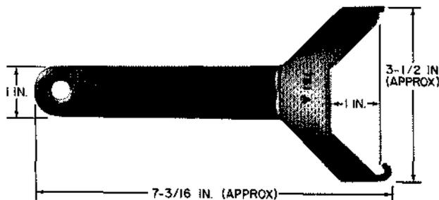
Extracting tool. For use in extracting or inserting plug-in units in the No. 4A and 4M Toll Switching Systems.
