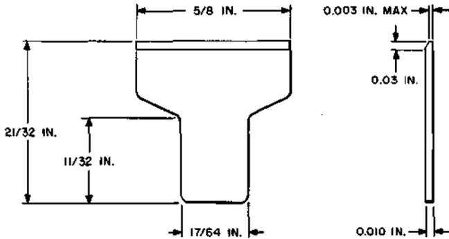
Insulator. For use in insulating the contacts during removal of the card from BF-, BG-, BJ-, and BL-type relays.
