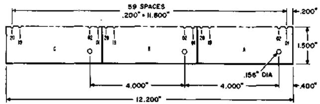
Locating and identifying tool. Used to locate and identify terminals for purposes of wiring and testing during manufacturing, installation, and maintenance. Initial use is on No. 101 ESS, J1H012A, and J1H013A switch units.
