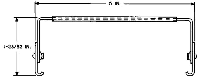
Extracting tool. The 748A tool was intended initially for use in extracting printed wiring board circuit packs of a data set in the No. 1 ESS.
