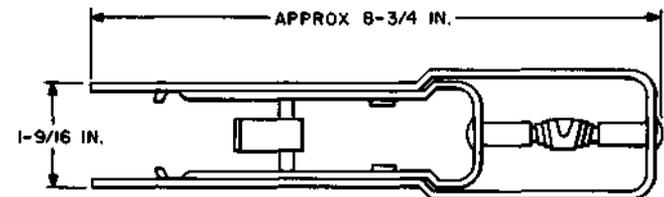
Extracting tool. For use in removing 89-type resistors from No. 1-type terminating sets.
