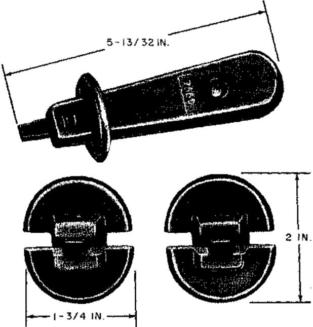
Connector tool. For use in seating 22 AWG IPVC wire in both single slip terminals and in quick-connect terminal welded assemblies on 78A and 78B connecting blocks on the ESS MDF.
