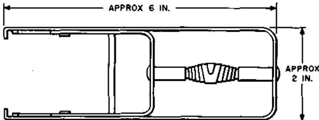
Circuit pack extractor. For use in removing D-type circuit packs from 910-type connectors.
