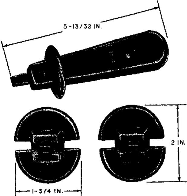
Connector tool. For use in seating 24 AWG IPVC wire in both single slip terminals and in quick-connect terminal welded assemblies on 78C-type connecting blocks on the COSMIC Frame System.
