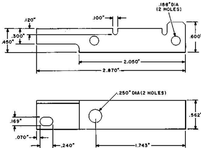
The 743A tool is used for locating a drilled hold necessary to modify coin collectors or coin telephones to accept a coin level detector.
