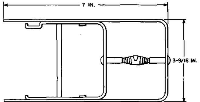
Extracting tool. For use in removing KS-19162 L14 plugs used on interconnecting switchboard cables between two No. 5 crossbar completing marker frames.
