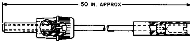
Test plug. For use in testing fuses in TD2 Radio Relay System.
