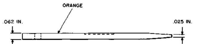
An orange-colored, wedge-shaped, blocking tool of insulating material. For use in blocking the HOLDING-OFF-NORMAL unit for the CA-CF types of small crossbar switches.
