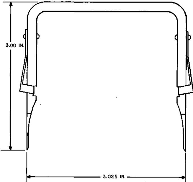
For use in removing 82A and 83A apparatus mountings.
