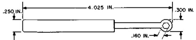
Torque wrench. For use with the 841282635 clamp.
