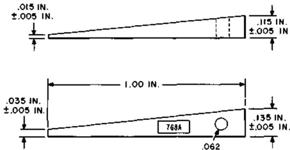
A plastic, orange-colored, wedge-type, blocking tool. For use in blocking the armatures of wire spring relays in the operated and unoperated positions. It may also be used to block operated or unoperated U-, UA-, UB-, and Y-type relays equipped with either the former nut or the new welded backstop and CA-CF type small crossbar switches. Replaces the KS-16887 L1 wedge and the 508A tool.
