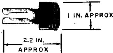
Locking tool. To lock the horizontal select bar on the CA-CF types of small crossbar switches.
