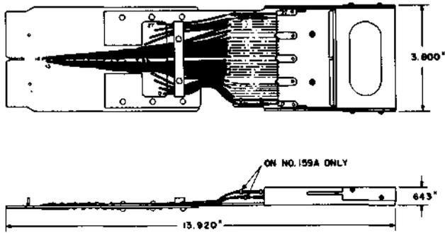
Each consists of a printed wiring board and a 905B connector assembled in a metal frame. The 158A has permanent connections between wiring board and the 905B connector. The 159A has connections between wiring board and the 905B connector which can be interchanged to permit a variety of tests. Intended for use in No. 1 ESS to permit printed wiring boards mounted in the 36A apparatus mounting to be extended beyond the apparatus mounting for testing purposes.
