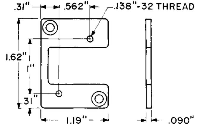
A metal U-shaped plate arranged to mount a 263A jack mounting in positions intended for mounting a 212A jack mounting. Intended for use in common systems.
