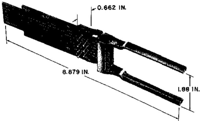
Consists of a printed wiring board equipped with test terminals, a 906F connector, and a U-shaped slotted metal guide bracket. Intended for use in testing D3 circuit packs.
