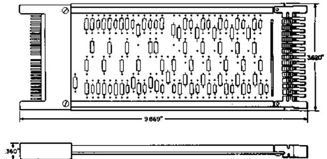
Consists of component apparatus mounted on a printed wiring board equipped with a P-42F226 terminal block on one end and a P37C859 connector on the other end. Initially used in No. 1 ESS.
