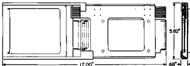
Consists of a steel framework equipped with sliding adjustable keys which mount into a 927-type connector. Intended for use in extending AR-coded circuit packs from their normal mounting positions in the 58A, 59A, and 61A apparatus mountings for in-circuit testing. Initially used in No. 1 ESS (ADF).
