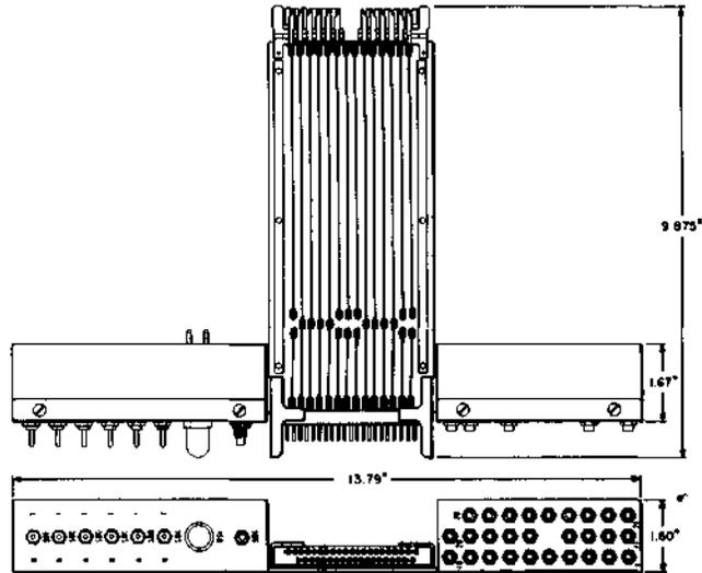
Consists of jacks, switches, and a lamp mounted on a metal mounting plate with terminal covers. A printed wiring board that contains eyelets used for plugging into the circuit is also assembled to the metal frame. Intended for use as an extender board and as an aid in locating faulty circuit pack of No. 1 ESS. Initially used in the 124A test set.
