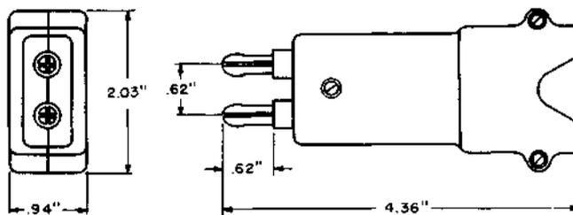
A twin plug and twin jack arranged for use with a 240 or similar-type jack and a 419A plug. Each finger provides sleeve contact only. Intended for use as a monitor plug adapter in E6 telephone repeaters of common systems.
