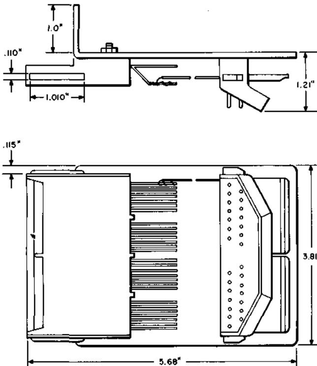
Consists of a printed wiring board and a 905B connector assembled in a metal frame. Intended initially for use in the No.1 ESS to permit testing of the trunk unit relays of the plug-in type trunk units.
