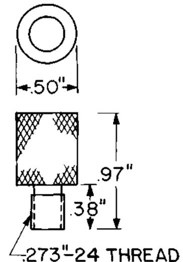
A metal adapter arranged to thread into a 413-type plug. Intended for use in testing cable pairs on main distributing frames equipped with 300-type connectors.
