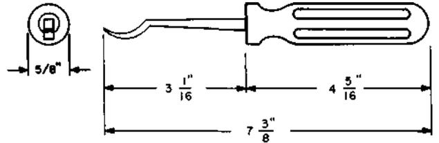
Jack ring spring adjuster. For use on the 92- and 292-type jacks.
