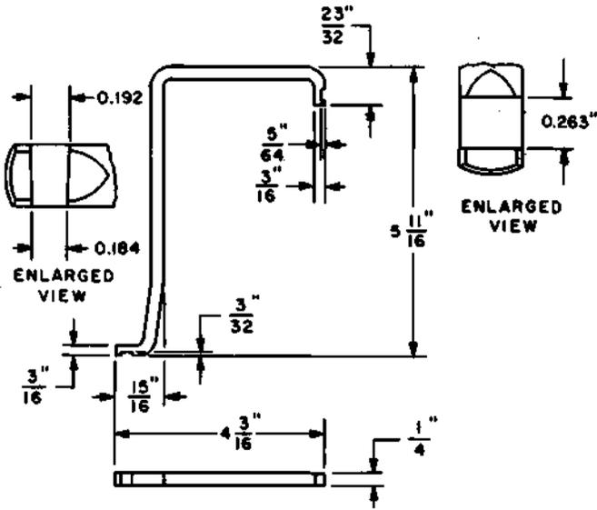
Replaces the 223 tool. For use on panel clutches, 197- and 198-type switches, and panel multiple banks.
