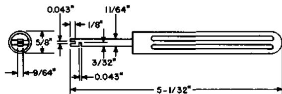
Retractable spring lug adjuster. For use on the 208- and 214-type relays.
