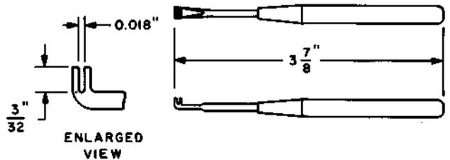
Spring adjuster. For use on precision-type interrupters and Stromberg Carlson relays.
