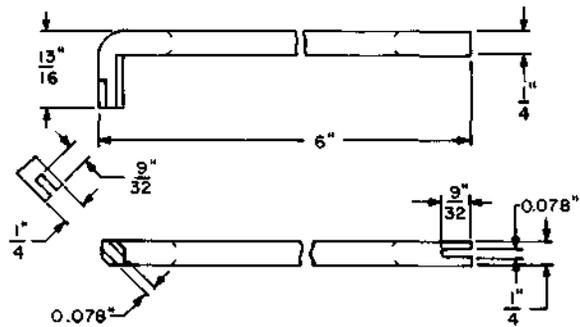
Replaces the 325 tool. For use on clutches, panel elevator apparatus, 200-, 204-, and 206-type selectors, and panel multiple bank guide combs.
