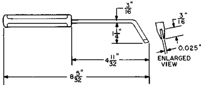
Spring adjuster. For use on 155A and 157-type interrupters, and A- and B-type and spring driven sequence switches.
