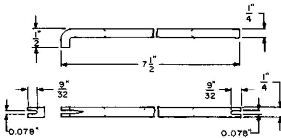
Replaces the 326 tool. For use on clutches, 50A drives, panel elevator apparatus, and L-, N-, and S-type relays.
