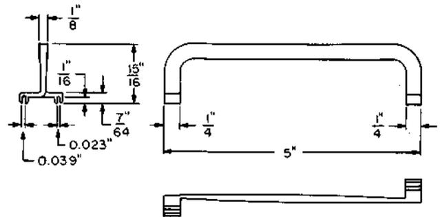
Spring adjuster. For use on round-type relays.
