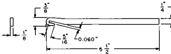
Guide adjuster. For use in adjusting 1-type guides.
