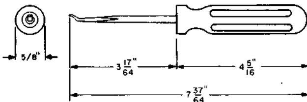
Jack tip and ring spring adjuster. For use on the 49-, 92-, and 292-type jacks.
