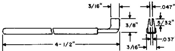
Spring adjuster. Replaces the 50 and 327 tools. For use on the 111- and similar-type relays and elevator apparatus.
