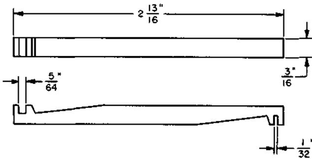
Spring adjuster. For use on the 197- and 198-type switches, 50-type dial testers, and power driven rotary selectors.
