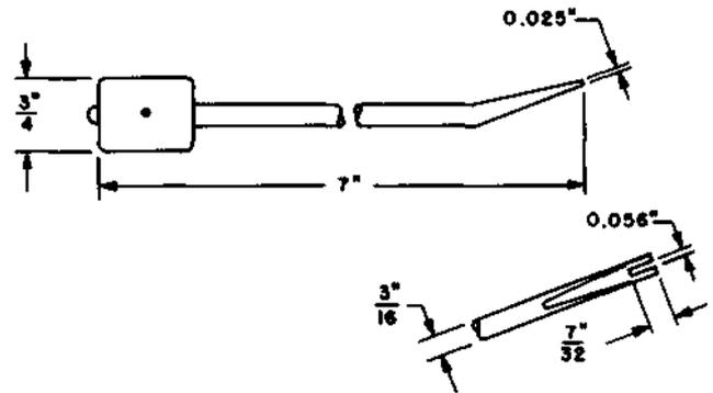
Spring adjuster. For use on panel elevator apparatus.
