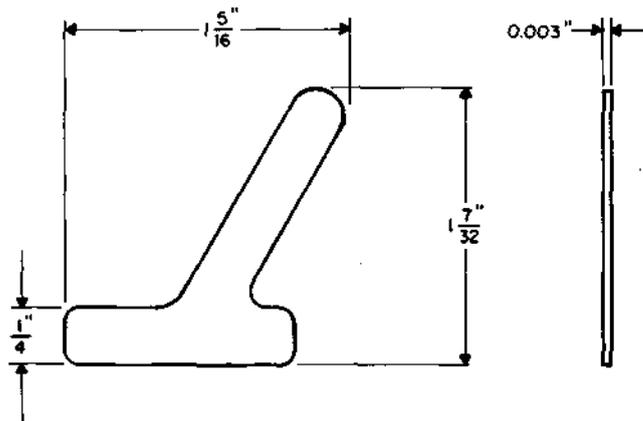
Heelpiece adjusting tool. For use on step-by-step type relays.
