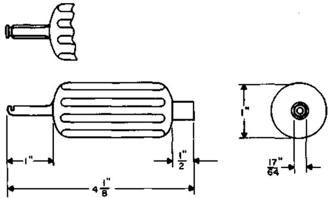
Protector wrench and adjuster. Replaces the 28 tool. For use on protector mountings and 444-type jacks.
