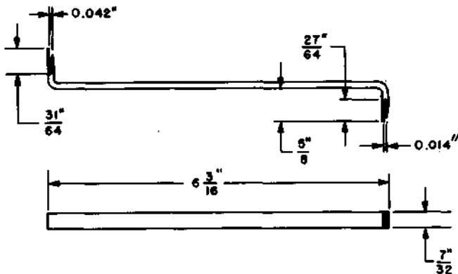
Replaces the 330 tool. For use on panel line finder, trunk finder, and call distributing "B" link elevator apparatus.
