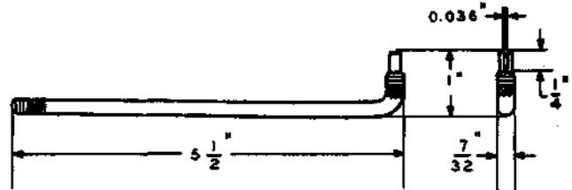
Spring adjuster. For use on 202-, 211-, and 212-type switches; and 229-, 230-, and 232-type relays.
