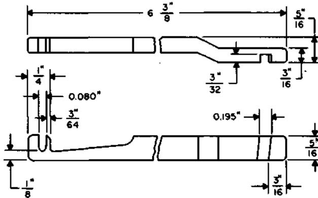
Replaces the 233 and 301 tools and adjuster R-63773. For use on helical spring-type clutches and 200- and 206-type selectors.
