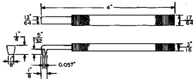
Spring adjuster. Replaces the 98 tool and the R-69710 spring adjuster. For general use.
