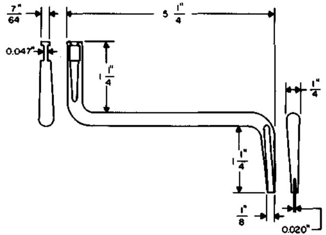
Spring adjuster. Replaces spring adjuster R-55760. For use on panel multiple brushes.
