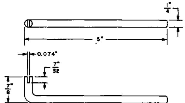
For use on 204-type selectors and 25-point rotary switches.
