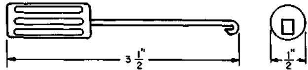
For use on 200- and 206-type selectors and power-driven rotary selectors.
