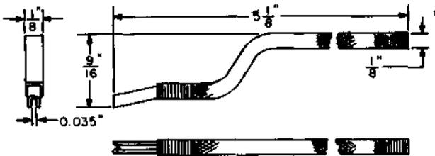
Multiple bank terminal adjuster. Replaces the 432A tool. For use on panel multiple banks.
