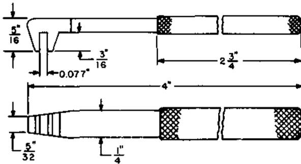
Spring adjuster. Replaces the D-178349 tool. For use in adjusting the retractile springs of KS-13835 readers.
