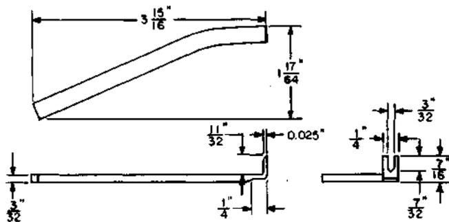
Spring adjuster. For use on gravity-type relays.
