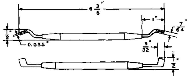
Spring adjuster. Replaces AECO spring adjuster H-20777 and the 416A tool. For use on relays, and 197-, 198-, 211-, 212-, and plunger-type line and out-trunk switches.
