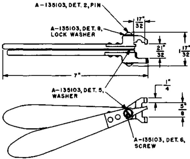
Front stop-lug adjuster. For use on 4-, 5-, 6-, and 7-type clutches.
