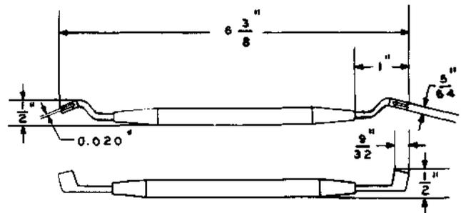
Spring adjuster. Replaces the 415A tool. For use on 197- and 198-type switches and step-by-step type relays.
