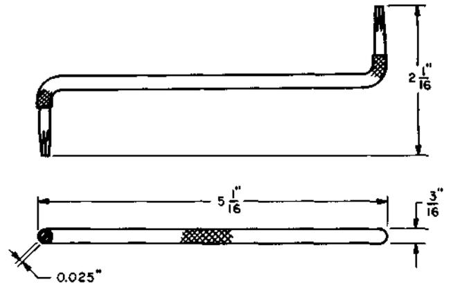
Spring adjuster. For use on split contact springs of A- and B-type sequence switches and 157-type interrupters.
