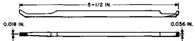
For adjusting cover spring on the AF-, AG-, AJ-, and AK-type relays.
