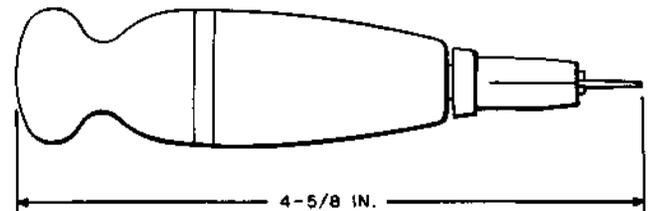
Six needles are furnished with each tool. For use on panel elevator apparatus.
