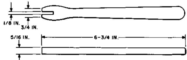
For use on solenoid-type master switches and plunger-type line and out-trunk switches.
