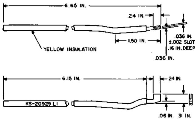
Replaces the 766A tool. Used for adjusting heavy springs and the armature backstop of the 221 FAE relays.
