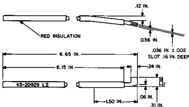
Replaces the 766A tool. Used for adjusting heavy springs and the armature backstop of the 221 FAE relays.
