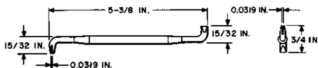
For use on step-by-step type relays and the 197- and 198-type switches.
