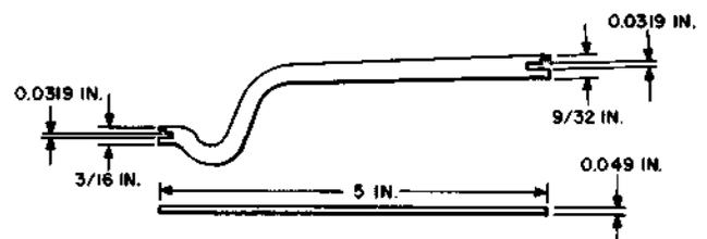
For use on step-by-step type relays.
