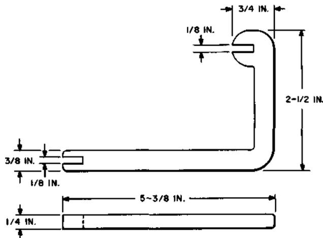
Replaces the AEC<sub>o</sub> H-7056 armature adjuster. For use on 197- and 198-type switches.
