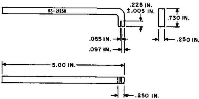
Used for adjusting the backstops of the U- and Y-type relays.
