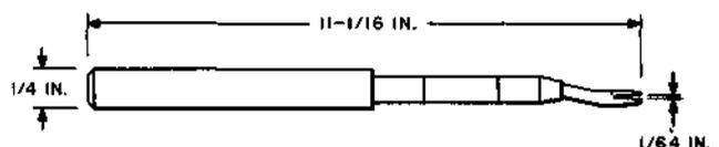
For use on plunger-type line and out-trunk switches.
