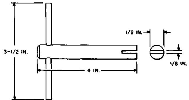
For use on plunger-type line and out-trunk switches.
