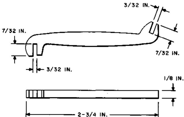
For use on 197- and 198-type switches and solenoid-type master switches.
