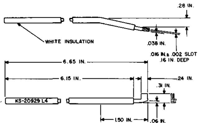
Replaces the 765A tool. Used for adjusting lower springs of the 221 FAE relays.
