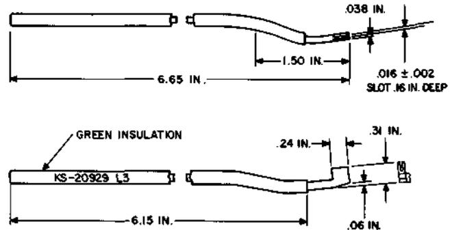
Replaces the 764A and 765A tools. Used for adjusting upper and lower springs of the 221 FAE relays.
