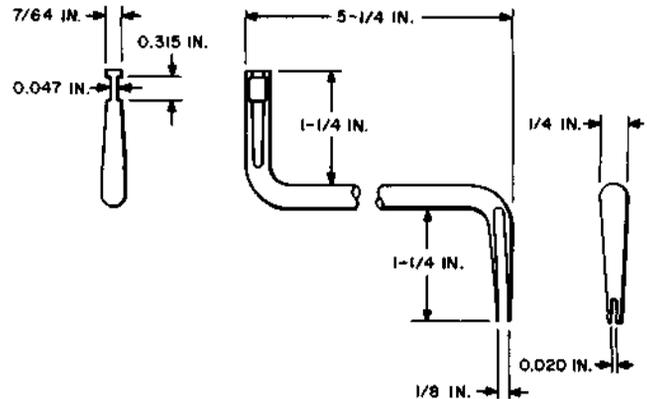
Similar to the 380A tool except that the openings shown at left in the above illustration are wider. For use on panel multiple brushes in cases where the 380A tool cannot be used because of brush springs being too wide.
