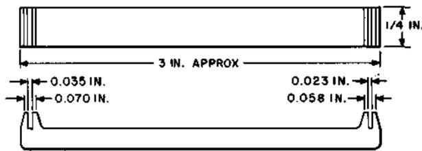
For use in adjusting normal post springs on the 197-type switches.
