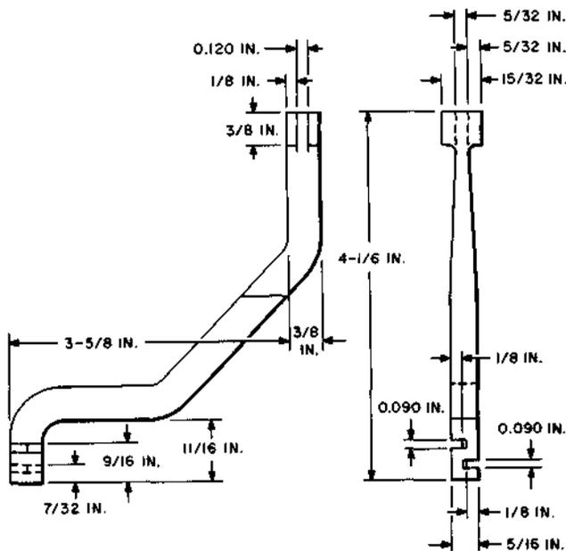
For use on the 200-, 206-, 209-, and 211-type selectors, 25-point rotary switches, and 1-type translators.
