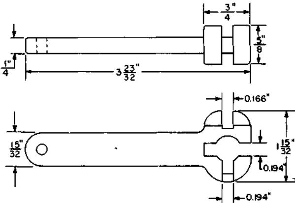
Wiper-shaft aligning wrench. For use on 197- and 198-type switches.
