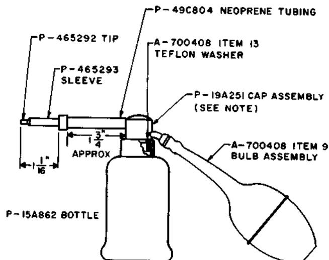
*Note:* When ordering the P-19A251 cap assembly, also order one A-700408 Item 13 Teflon washer. Thread washer on cap before mounting cap on bottle.
