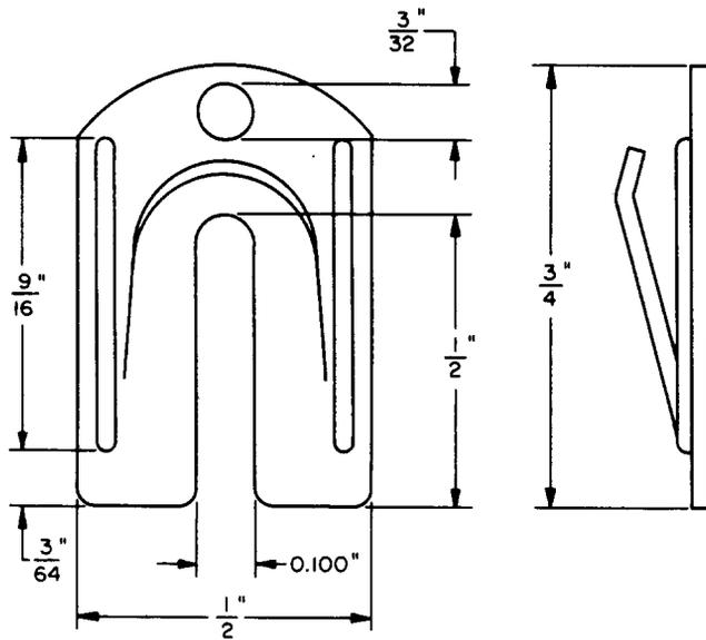
Relay blocking tool. Replaces the 136 tool. For use on certain flat-type relays.
