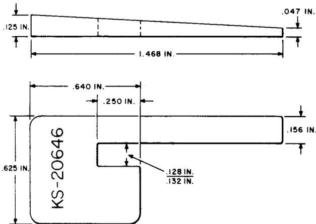
Wedge. For use in blocking the selecting bar of CA-through CF-type small crossbar switches. Colored fluorescent orange.
