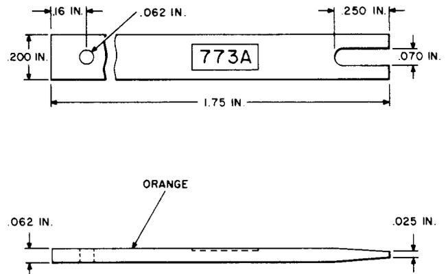
A wedge-shaped blocking tool of insulating material. For use in blocking the HOLDING-OFF-NORMAL unit for the CA- through CF-type small crossbar switches.
