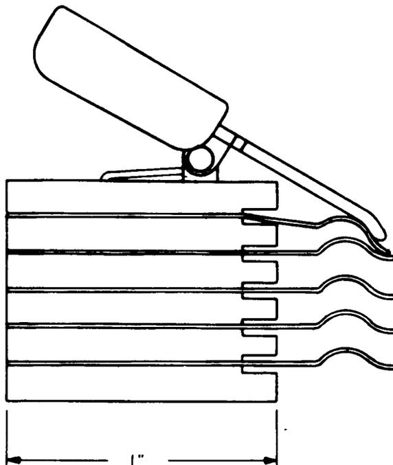
Spring blocking tool. Replaces the D-170030 spring blocking tool. For use in replacing cards on 304- and similar-type switches.
