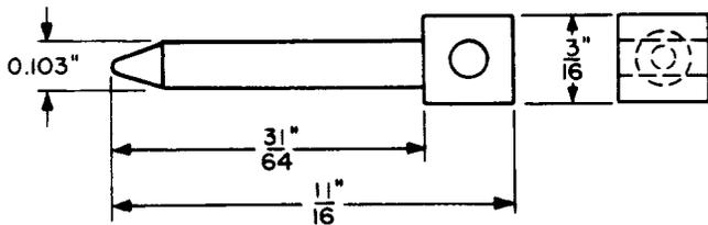
Cutover tool. For use on 300- and similar-type switches. Replaces the 550A tool.
