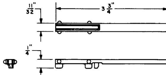
Armature blocking tool. For use on 300- to 308-type, 314, 315-, and 318-type switches. Replaces the 542A tool.
