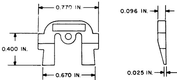
Wedge. For blocking BF-, BG-, BJ-, and BL-type relays in either operated or unoperated positions.
