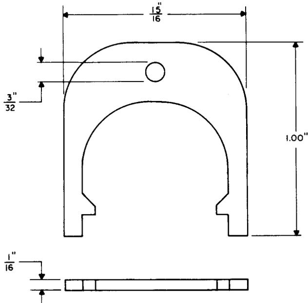
Contact blocking tool. For use in blocking the contacts of the EA1 relay which control the circuit through the line relay in 701B PBX installations.
