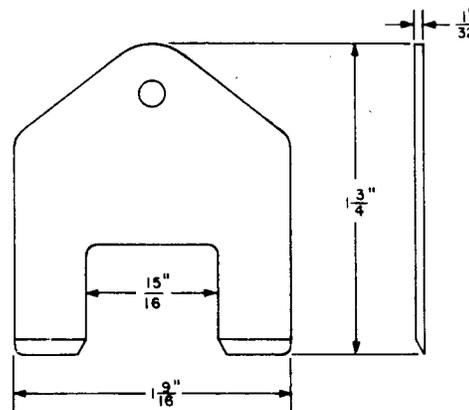
Cutover tool. For use on U676 and U680 relays in step-by-step dial systems.
