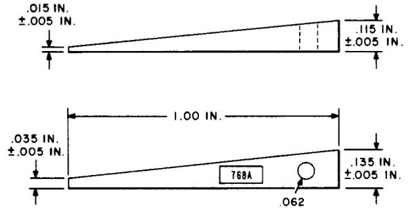
A plastic, wedge-type blocking tool. For use in blocking the armatures of wire spring relays in the operated and unoperated positions. It may also be used to block operated or unoperated U-, UA-, UB- and Y-type relays equipped with either the former nut or the new welded backstop and CA- through CF-type small crossbar switches. Replaces the 508A tool. Colored fluorescent orange.
