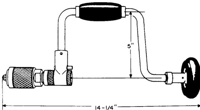
Jaws take square bit stocks up to 5/8-inch across corners and straight or tapered shanks up to 1/2-inch in diameter. Replacement parts listed below may be ordered:
