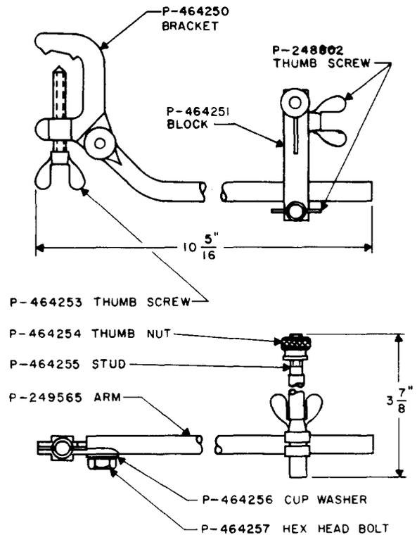
Gauge positioning bracket. For use in checking reciprocating bar-type interrupters.
