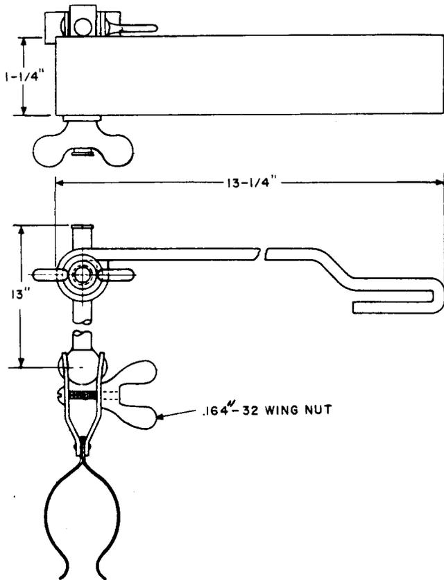
Designed to hook over the top angle of step-by-step switch shelves. The bracket has an adjustable arm for holding a portable lamp guard in various positions. For use in checking and adjusting step-by-step switches and associated apparatus.
