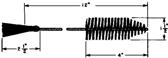
A bottle-type typewriter brush having a twisted wire handle 12 inches long. For use on friction roll drives and plunger-primary and secondary line and out-trunk switches.
