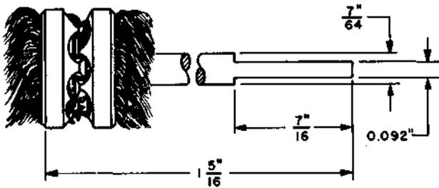
Replaces but not interchangeable with the 133 tool (spring cleaning tool). For use in conjunction with 1495 WE all-angle drill.
