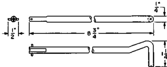
Bumper. Replaces R-80215 bumper. For use on plunger-type line switches.
