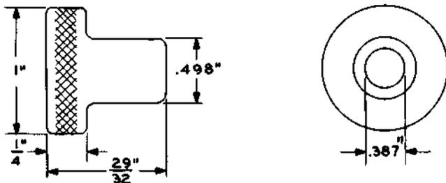
Tapered bushing. For use with the D-97083 reamer for reaming bearings in worm case housings of friction roll drives
