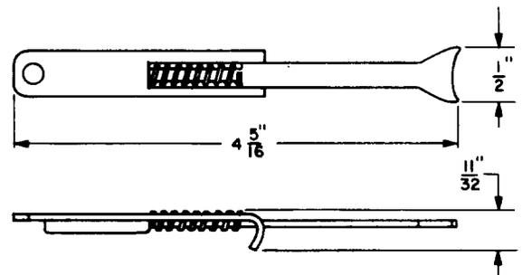
Make-busy tool. For grounding the outside springs of 245-, 254-, 263- and 264-type relays by shorting the springs to the cover ground. On 245- and 254-type relays, the tool clamps on the spring. On 263- and 264-type relays, the tool clamps on the insulator which forces the tool prongs against the spring. Replaces the 530A tool. For use on 245-, 254-, 263- and 264-type relays.
