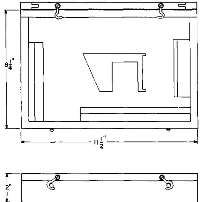
A gray-finished wooden case with a hinged cover held closed by a latch. Part of the 1014B tool kit and used for housing the tools of that kit.
