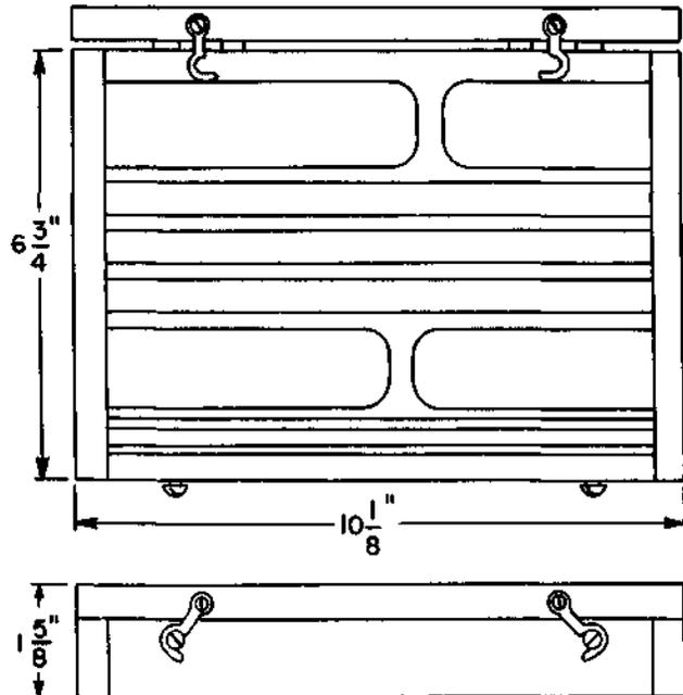
A black-finished wooden case with a hinged cover held closed by a latch. Part of the 1002A tool kit and used for housing tools of that kit.
