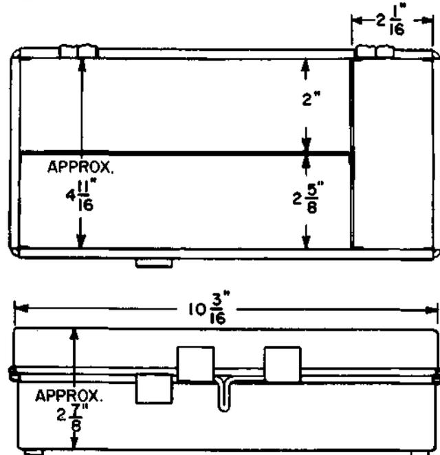
A black-finished sheet metal case with a hinged cover held closed by a latch. The interior is divided into three compartments. For housing and carrying multiple marking tools and materials.
