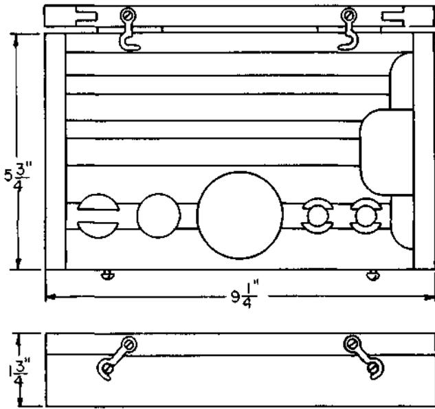
A black-finished wooden case with a hinged cover held closed by a latch. Part of the 1000A tool kit and used for housing the tools of that kit.
