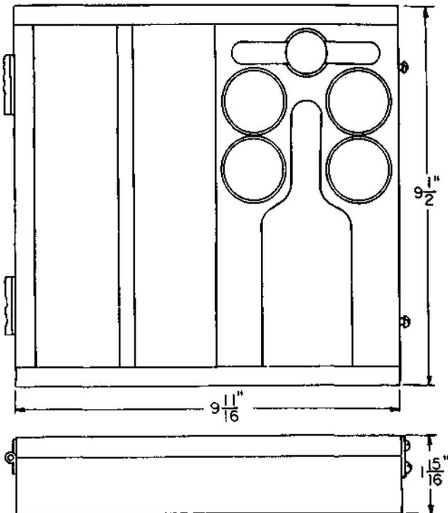
A black-finished wooden case with a hinged cover held closed by a latch. Part of the 1001A tool kit and used for housing tools and gauges of that kit.
