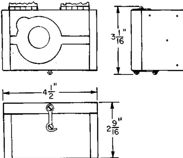
A black-finished wooden case with a hinged cover held closed by a latch. For housing and carrying the 121A gauge.
