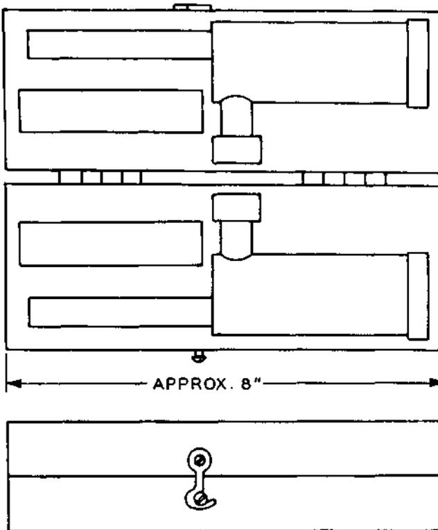
A black-finished wooden case with a hinged cover held closed by a latch. Part of the 1003A tool kit and used for housing tools of that kit.
