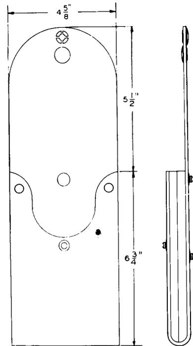
Fig. 1—AT-6475 Pocket Tool Case
