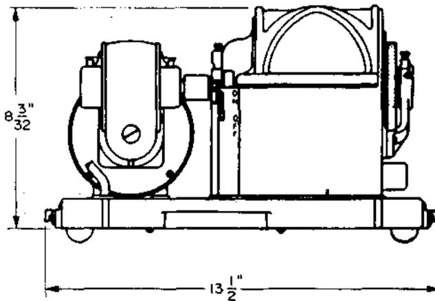
Plug cleaner. The 497A tool is for ac operation. Intended for use in cleaning plugs at telephone switchboards. The 498A, 498B, and 498C tools are required for use with this plug cleaner.
