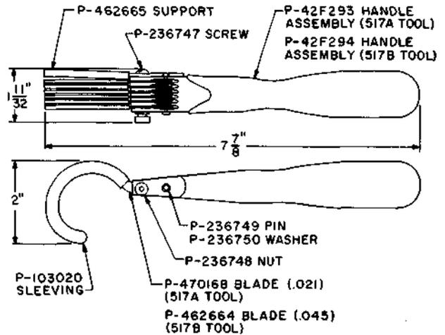
Bank contact cleaners. The blades and support of the 402E tool may be used in the handle of the 517A tool. The 517A tool replaces the 402D tool and is used in cleaning the contacts of 200-point banks of 197-type switches. The 517B tool is used in cleaning the contacts of 100-point banks of 197-type switches and 40-point banks of 198-type switches.
