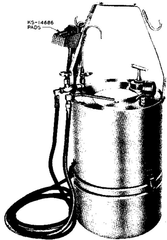
Mounts three KS-14686 pads which are arranged to scrub six cam sides simultaneously. The pads must be ordered separately. Refer to Section 069-601-801 for piece-part data and maintenance information for this tool. Replaces the 435A tool. For use in cleaning cams of sequence switches and 157-type interrupters.
