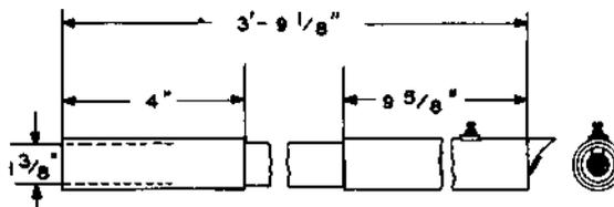
Consists of a fiber tube nozzle and a 3-foot long flexible hose. Furnished with one KS-3093 brush. For use on 153-type interrupters.
