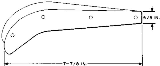
For use in cleaning plunger-type line switch springs.
