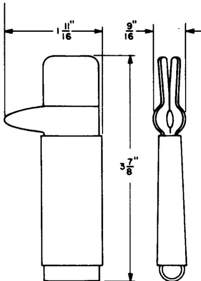
Cushion placing clip. Used in conjunction with 515A tool. For placing 1A and 2A cushions on 109, 309, 110, or 310 plugs. Also for placing 4A cushions on 47- or 347-type plugs. Replaces the KS-7872 pliers.
