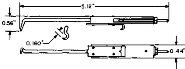
Relay winding connector. Replaces the 428A tool. For use in making test connections from the front of the relay on 89-, 101-, 105-, 108-, 111-, 121-, 122-, 149-, 162-, 172-, 178-, 179-, 190-, and 196-type relays.
