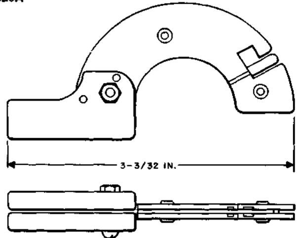
Bank contact connector. For use in making test connections to the bank contacts of step-by-step line finder switches. A W3AJ cord is required for connecting this tool.
