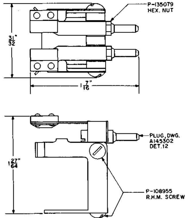
Intercontact connector. For use on 111-type relays.
