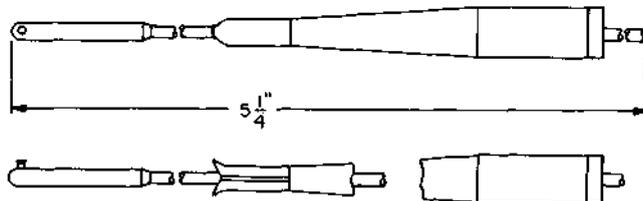
Relay winding connector. For use with a 360-type tool to connect to winding terminals of U-, Y-, and similar-type relays, and 263- and 264-type relays.
