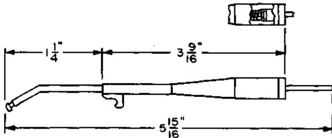
Magnet winding connector. Used in conjunction with the 360-type tool. For use on 300- and similar-type switches.
