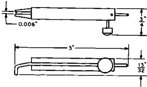
Test connector. Replaces the 252 tool. For use in making test connections to A- and B-type sequence switches, 157-type interrupters, and relays.
