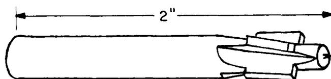
For use in replacing springs and studs of Dzus fasteners.
