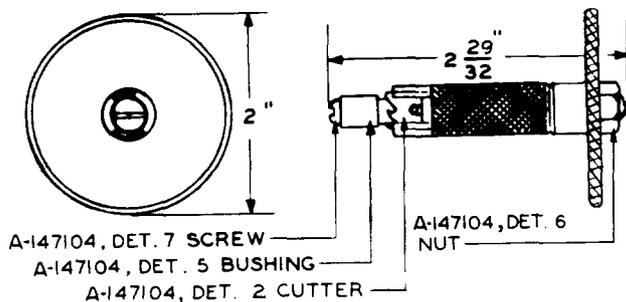
Jack mounting counterbore. For counterboring jack mounting to accommodate the shoulder of a replacement sleeve for worn 141-type jacks.
