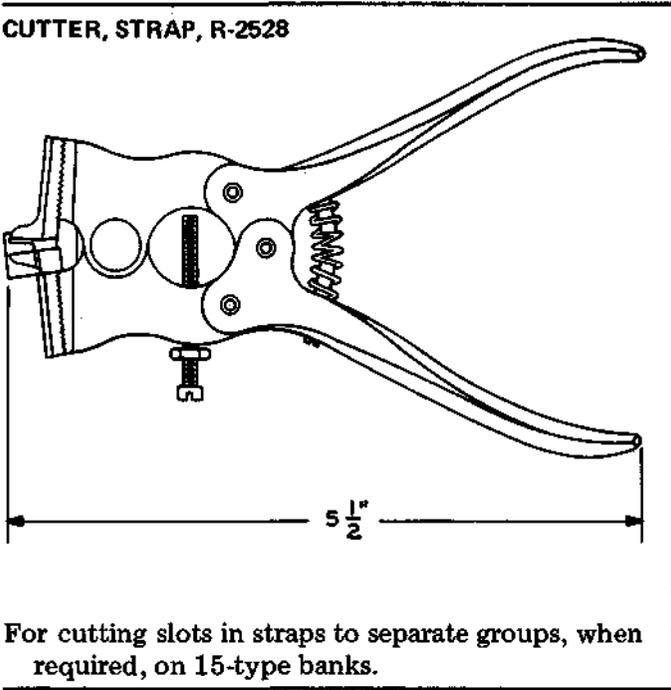
For cutting slots in straps to separate groups, when required, on 15-type banks.
