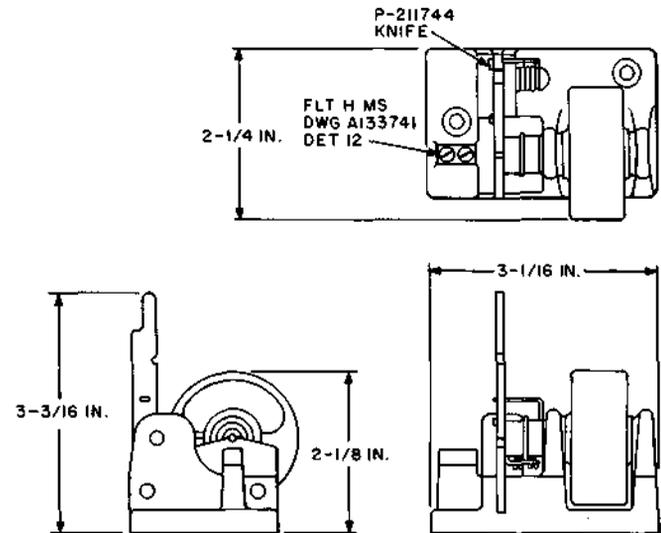
Conductor braid cutter. For use in repairing switchboard cords by the punched-hole method. The information covered herein replaces the part of Section 074-000-006, Issue 1, applying to this tool.
