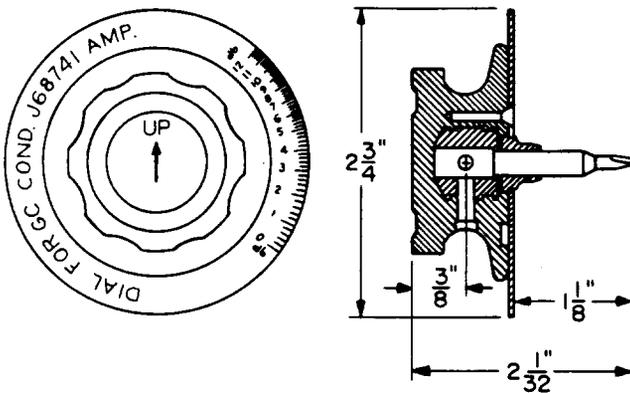
Screwdriver dial. For use in adjusting gain of type K carrier line amplifier J68741A.
