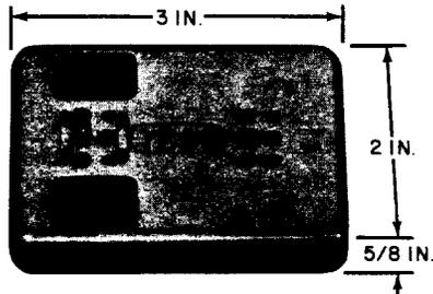
Disassembly fixture. A small plastic panel which provides a plug-in position for both types of 3A and 4A protector units. One position is arranged for the older type units and the other position is arranged so that the snap-on housing of the 3A5A and 4A5C protector units may be easily removed. Intended for use in repairing those protector units at central office locations. Replaces 760A tool.
