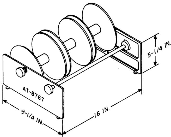
The B wire dispenser is a plastic supporting device for three 267C-type metal spools (not supplied) placed in tandem on a common rod. It is equipped with a spring-loaded clutch to prevent overfeeding of the wire. Orders should be worded as follows:
