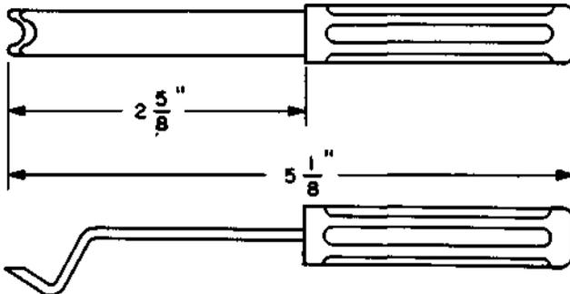
Signal plug extractor. For use in extracting signal plugs from multiple jacks and 350A make-busy plugs at outgoing trunk test frame.
