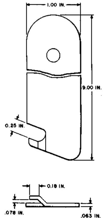
Signal unit extractor. For use in disengaging E-type signal units from their frame connectors.
