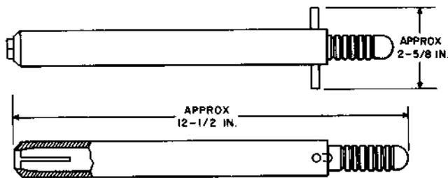
For use in extraction and insertion of 51A pads in L4 Coaxial System.
