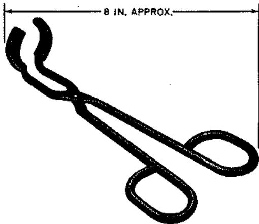
Tube extractor. For use in extracting the 375A and similar-type octal base electron tubes and for removing and replacing 89-type resistors.
