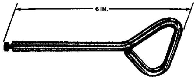
For use in removing packaged semiconductor amplifiers from L-type multiplex equipment.
