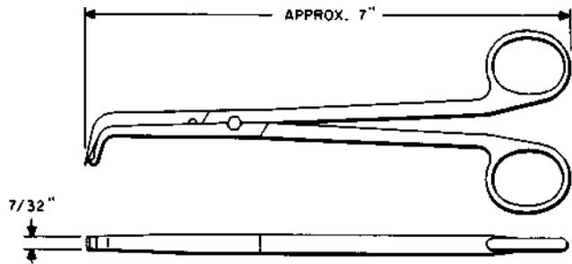
Pin extractor. For use in removing and replacing pins in KS-13882 perforators in AMA accounting centers and central offices.
