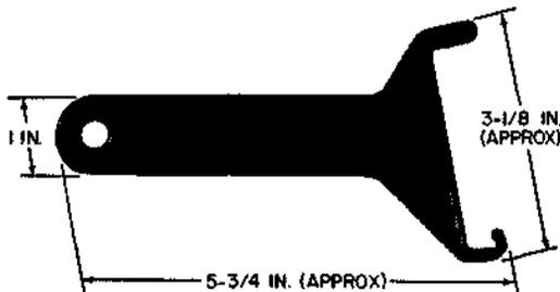
Tube extractor. For use in extracting 373A and 374A electron tubes from K2 carrier telephone equipment panels.
