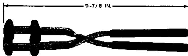
For use in extracting 310- and 311-type electron tubes.
