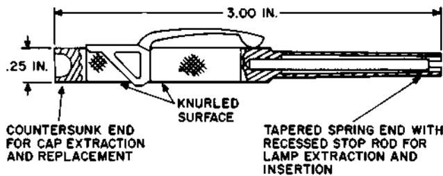
Lamp and cap extractor. A double-ended tool used to remove the cap and T1-type lamp from the miniature lamp assemblies used in L4 and L5 terminal equipment. Refer to Section 075-126-301 for details and use.
