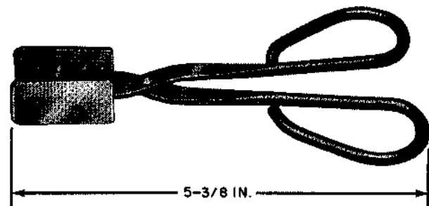
For use in removing the 372A and similar-type patching plugs from the A2A Video System.
