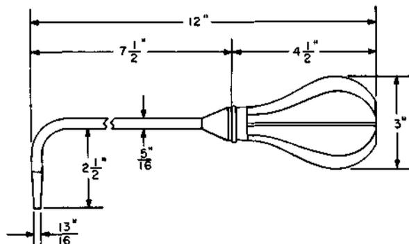
For use on KS-5361 L100, L110, L111, L112, L113, L114, and L115 batteries.
