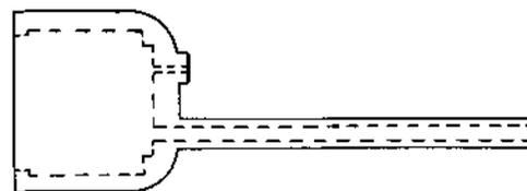
Consists of a rubber stopper having a spout and air hole. To be mounted on a bottle of about 1 quart capacity. For use in adding distilled water to storage battery cells.
