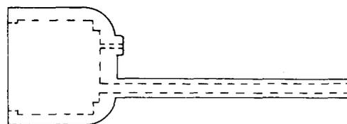
Consists of a rubber stopper having a spout and airhole. To be mounted on a bottle of about 1 quart capacity. For use in adding distilled water to storage battery cells.
