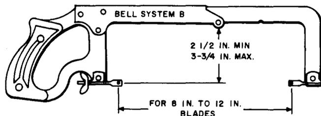
The B hacksaw frame accommodates 8-inch to 12-inch hacksaw blades. Blades for hacksaw frame must be ordered separately. See Blades, Hacksaw, for lengths and teeth per inch. For general use.
