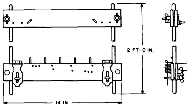
For use in connecting conductors at terminal strips.
