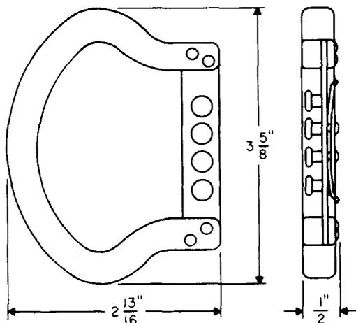
Hand grip. For use in cleaning rotor hubs of 200-, 206-, 209-, and 211-type selectors and 25-point rotary switches.
