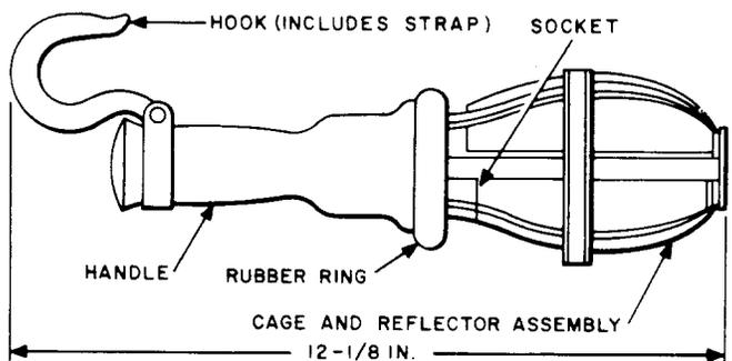
Consists of a kit of parts to be assembled in the field as a "trouble" light. Parts supplied are a soft rubber handle, fiber cage and reflector assembly, lamp socket, and fiber hook. When assembled to a suitable cable, the light is intended for general 120 Vac use.
