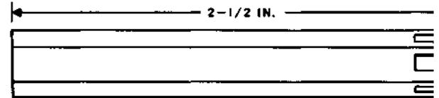
Drill guide. For use in removing rivets of D: fasteners.
