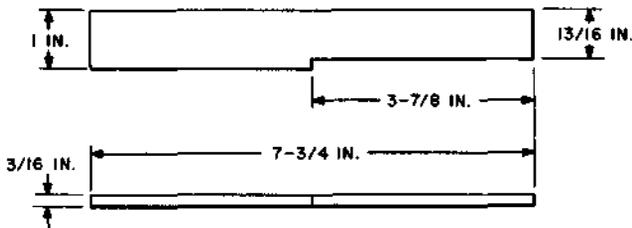
For use in replacing worn contact springs of sequence switches.
