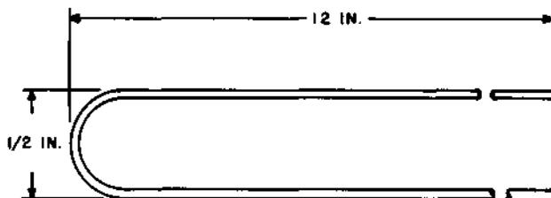
Hairpin guide. Used as an aid for replacing defective hairpin select wires with the vertical units of a small crossbar switch mounted in an equipment frame.
