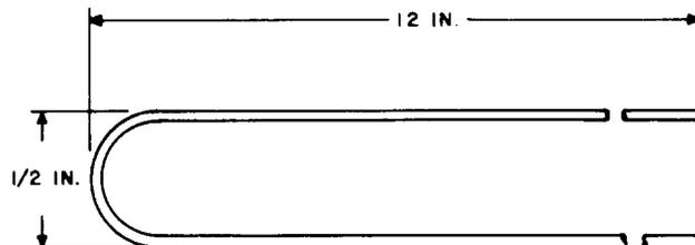
**Hairpin Guide.** Used as an aid for replacing defective hairpin select wires with the vertical units of a small crossbar switch mounted in an equipment frame.
