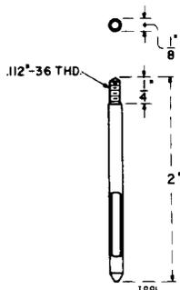
For use as an aligning guide to facilitate mounting No. 4 and 5 type dials on coin collectors.
