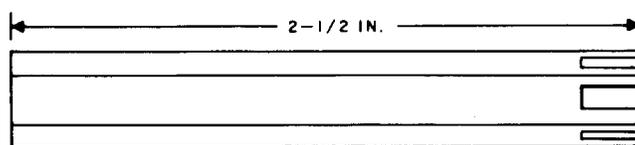
**Drill Guide.** For use in removing rivets of Dzus fasteners.
