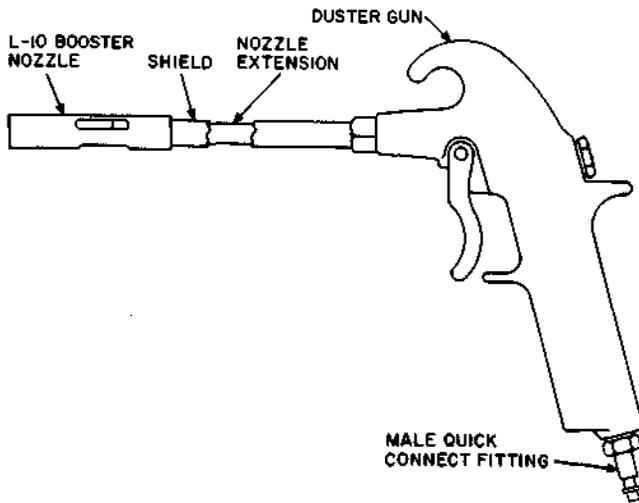
Duster gun. For use with KS-21231 L1 compressor set which replaces the KS-14514 L2 compressor set used for central office cleaning.
