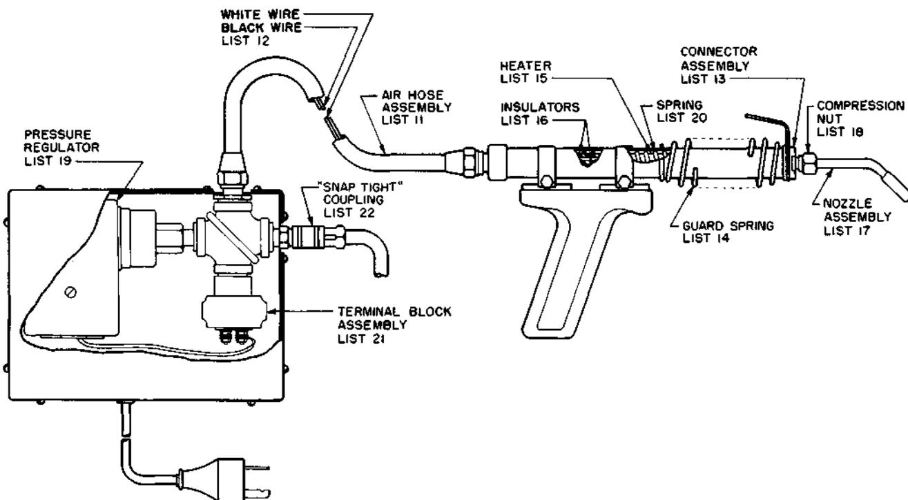
Hot-air gun. Consists essentially of a gun, an air-hose and a current control unit. Operates on 115 volts ac or dc with a power consumption of 300 watts.
