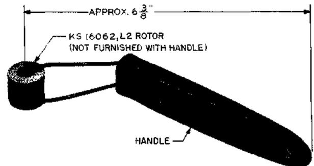
Handle having spring yoke for holding bank cleaning rotor. The KS-16062 L2 rotor used in this tool must be ordered separately. For use in cleaning step-by-step bank contacts and separators.
