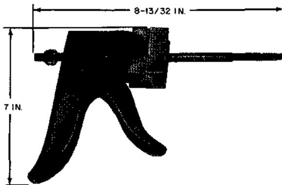
Ratchet handle. This tool forms part of 1014B tool kit. For use in conjunction with 716A and B tools when replacing coils of AF-, AG-, AJ-, and AK-type relays.
