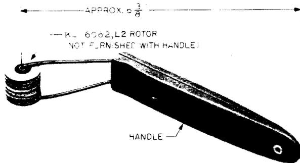
Handle having spring yoke for holding bank cleaning rotor. The KS-16062, L2, rotor used in this tool must be ordered separately. For use in cleaning step-by-step bank contacts and separators.
