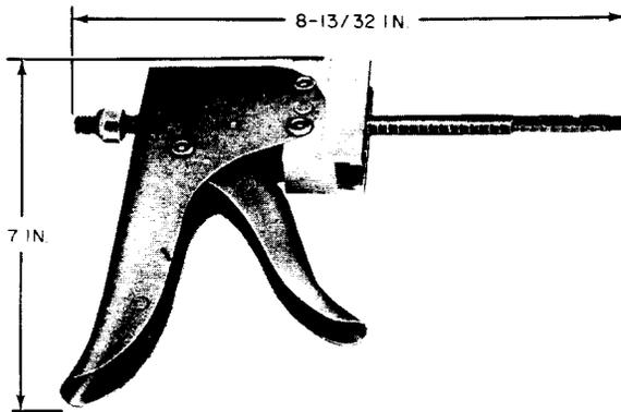
**Ratchet Handle.** This tool forms part of the 1014B tool kit. For use in conjunction with 716A and B tools when replacing coils of AF-, AG-, AJ-, and AK-type relays.
