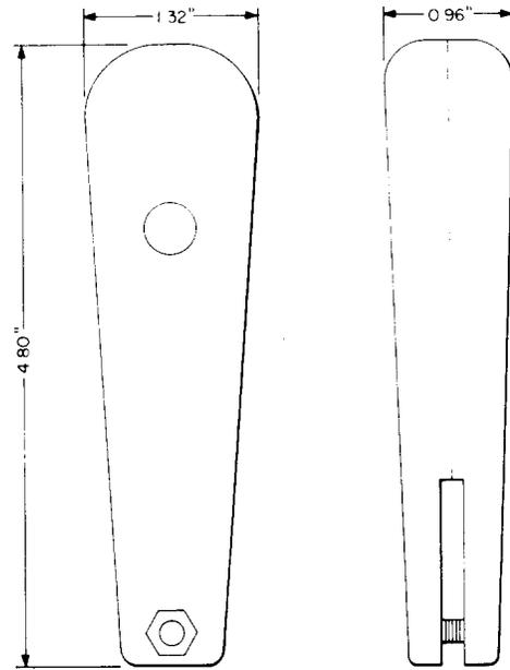
A two-piece plastic handle arranged to accommodate a No. 788 type tool for use on No. 88 type connecting blocks.
