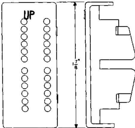
Relay contact connector holder. For use in conjunction with the 639A and 360-type tools for making connections to the fixed contacts on 24-position AJ-type relays.
