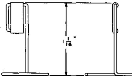
Spring holder. For holding movable springs in positions 13 to 18 when replacing cards on 24-position AJ-type relays.
