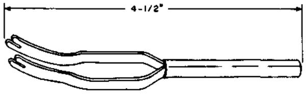
Multiple strip holder. For use in supporting the front multiple contact strip on vertical units of the 324-, 325-, and 328-type crossbar switches.
