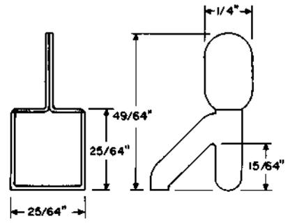
Spring holder. For use in holding the left row of movable contact springs when replacing stationary contacts of 286-, 287-, and 288-type relays.
