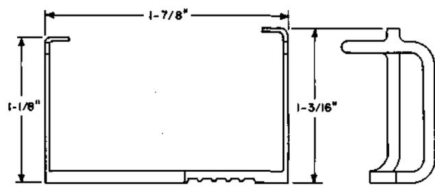
Spring holder. For holding the movable make contact springs when replacing cards or stationary contacts on the lower half of AK-type relays.
