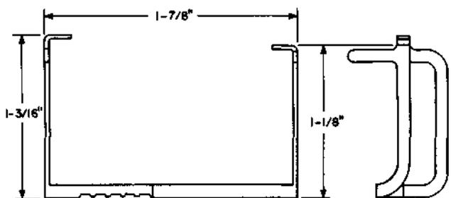
Spring holder. For holding the movable make contact springs when replacing cards or stationary contacts on the upper half of AK-type relays.
