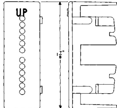
Relay contact connector holder. For use in conjunction with the 639A and 360-type tools for making connections to the fixed contacts on AF-, AG-, and 12-position AJ- and AK-type relays equipped with a contact cover spring.
