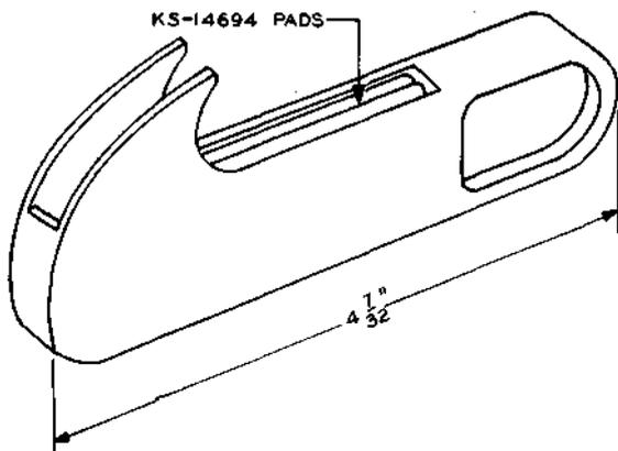
Scouring pad holder. The KS-14694 pads used in this tool must be ordered separately. For use in scouring sequence switch cams.
