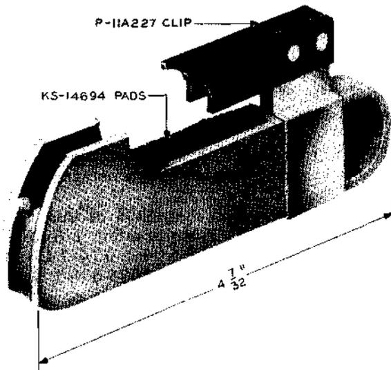
Scouring pad holder. The KS-14694 pads used in this tool must be ordered separately. For use in scouring sequence switch cams where equipment arrangements are such that the 653A tool can not be used.
