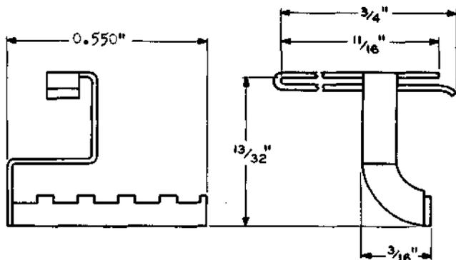
Spring holder. For holding the movable break contact springs when replacing cards or stationary contacts on the upper half of AK-type relays.
