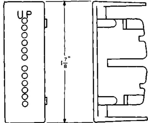
Relay contact connector holder. Used only on the initial production (less than 100,000) 12-position relays which were equipped with covers having metal frames. It is not satisfactory for use on any other relays. For use in conjunction with the 639A and 360-type tools for making connections to the fixed contacts on AF-, AG-, and 12-position AJ-type relays not equipped with a contact cover spring.
