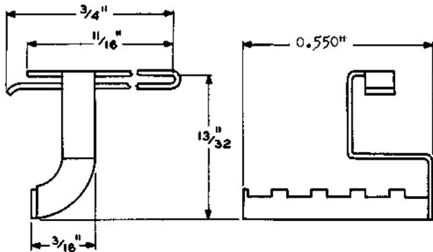
Spring holder. For holding the movable break contact springs when replacing cards or stationary contacts on the lower half of AK-type relays.
