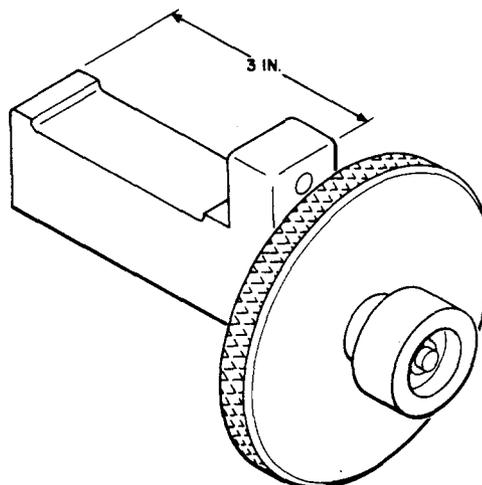
Consists of a shaped block, a knurled knob, and a threaded rod. For use on the 1A card writing unit. (Used initially in No. 1 Electronic Switching System.)
