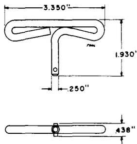
Used to release the housing and door locking mechanisms of the No. 1A type coin telephone sets after first opening the locks with keys.
