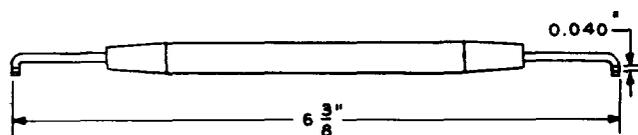
Balancing spring lifter. For use in disengaging the balancing spring from the card on AF-, AG- and AJ-type relays.
