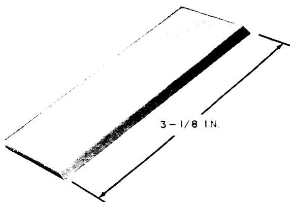
Spring lifter. This tool forms part of the 1012A tool kit. For use in replacing cards of 286-, 287-, and 288-type relays.
