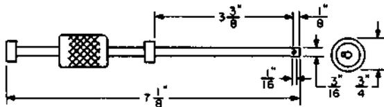
Cam locating tool. For use on 155A and 157-type interrupters and A- and B-type sequence switches.
