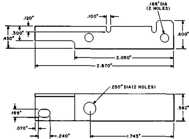
The 743A tool is used for locating a drilled hole necessary to modify coin collectors or coin telephones to accept a coin level detector.
