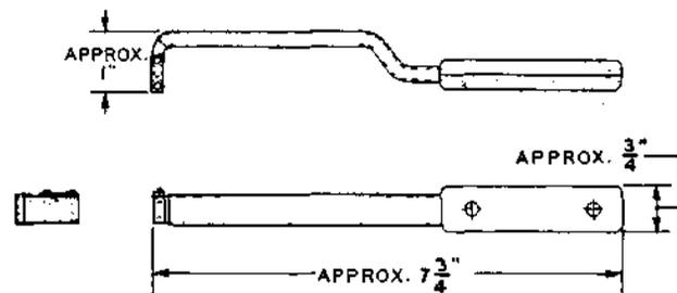
Commutator brush guide mounting tool. For use in installing rear guides on panel commutator brushes.
