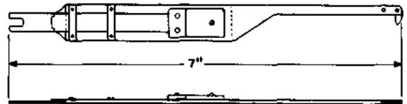
Operating spring stud cap mounting tool. For use in removing and replacing operating spring stud caps on worn studs of 245-, 254-, 263-, and 264-type relays.
