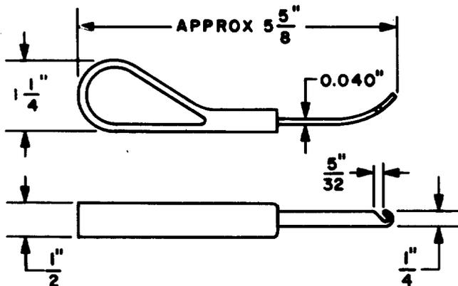
Curved cable sewing needle. For use in sewing local cable (PBX installation only).
