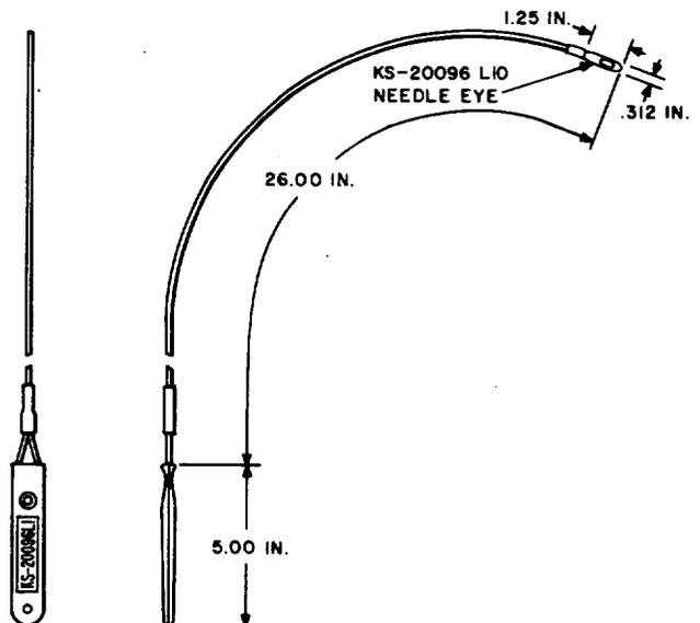
A curved, insulated, metal rod equipped with an insulated eye at one end arranged to thread four 22-gauge insulated wires. The other end is provided with an insulated handle. The KS-20096 L10 needle eye may be ordered as a separate item to replace damaged eyes on KS-20096 L1 needles in the field. For use in running jumpers on the No. 1 ESS main distributing frame.
