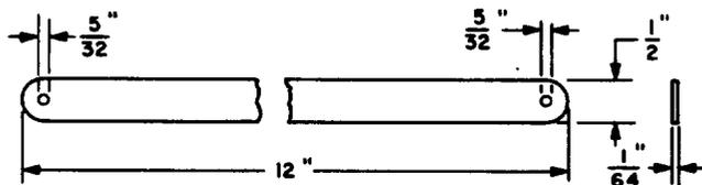
Straight cable sewing needle. For use in sewing local cable (PBX installation only).
