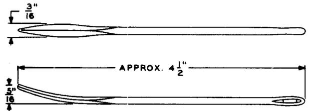
Sack needle. Steel needle for use in sewing cable forms (PBX installation only).
