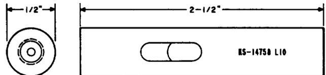
Booster nozzle. This tool forms part of the KS-14758 L2 duster gun. For use in central office equipment cleaning.
