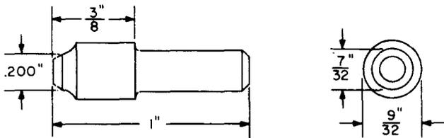
Hardwood pin. For use in conjunction with portable motor equipment for base metal contact maintenance in cleaning flared portion of 92- and 292-type jack sleeves.
