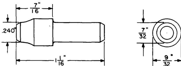
Hardwood pin. For use in conjunction with the portable motor equipment for base metal contact maintenance in cleaning flared portion of 49-type jack sleeves.
