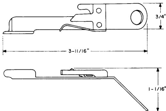
Brake plate. Replaces the 253 tool. For use on A- and B-type sequence switches.
