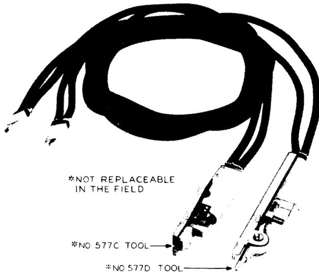
**Welding pliers** equipped with 57-inch leads. Forms a part of the 1013A tool kit. For use in replacing contacts on wire spring relays.
