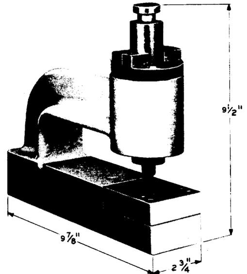
Tab-clipping punch and die assembly. This tool forms part of the 659E tool.
