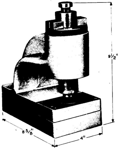
Hole-enlarging punch and die assembly. This tool forms part of the 659E tool.
