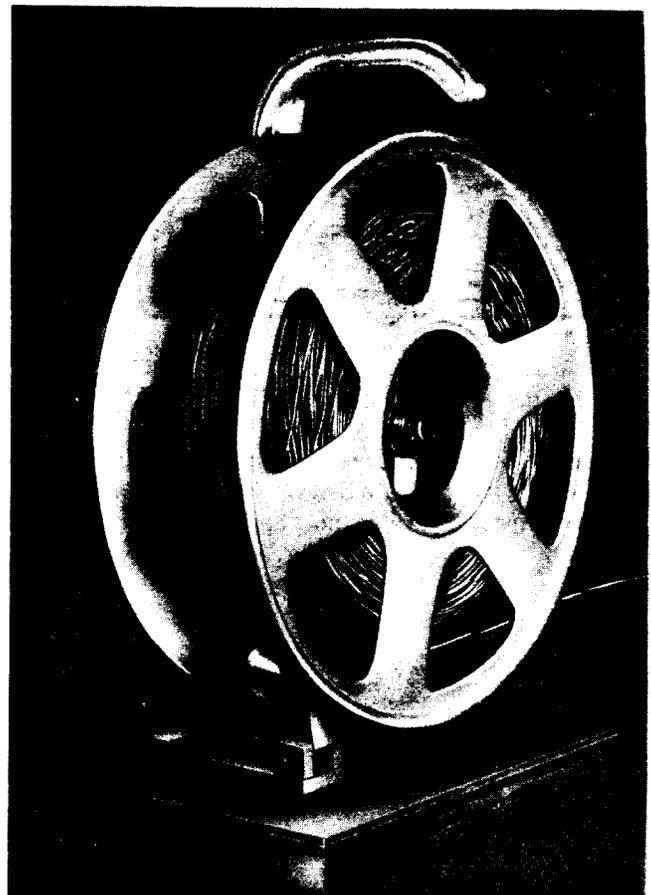
For use in central offices for holding distributing frame wire. This reel will be temporarily retained for maintenance and special requisitions. Replaced by the KS-21955, L1 wire reel.
