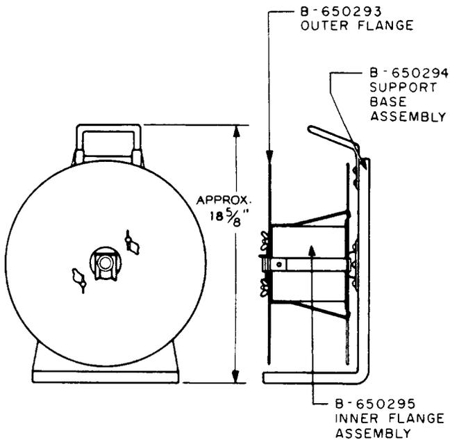
For use in central offices for holding distributing frame wire. The KS-8289 wire reel has been Mfr Disc. There is no replacement.
